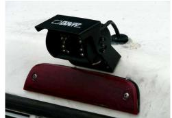
Figure 5. Camera mounted just above top rear brake light.
