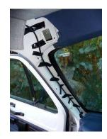
Figure 9. Run the camera cable down the A-pillar and secure it with electrical tape.
