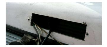
Figure 2. Top brake light hole allows cable fishing from inside.
