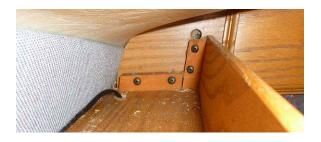
Figure 8. Camera cable runs down through tray front into A-pillar behind cloth trim.
